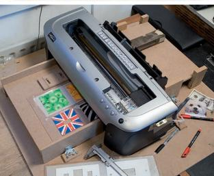
straight-through flatbed printing onto a 2mm thick metal plate.
