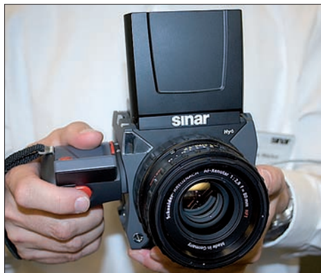
ABOVE LEFT AND RIGHT: Leaf Aptus 75 back mounted on a mock-up of the forthcoming Jenoptik body. BELOW LEFT AND RIGHT: Sinar eMotion 75 back mounted on a mock-up of the forthcoming Jenoptik body.
