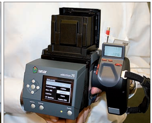
ABOVE LEFT AND RIGHT: Leaf Aptus 75 back mounted on a mock-up of the forthcoming Jenoptik body. BELOW LEFT AND RIGHT: Sinar eMotion 75 back mounted on a mock-up of the forthcoming Jenoptik body.
