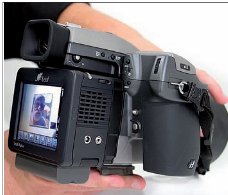
ABOVE: Leaf's studio setup at Photokina showed the many different configurations for the Aptus 75 back. BELOW LEFT: LEaf Aptus 75 back mounted on Hasselblad H2 body. BELOW RIGHT: On the new Jenoptik body.
